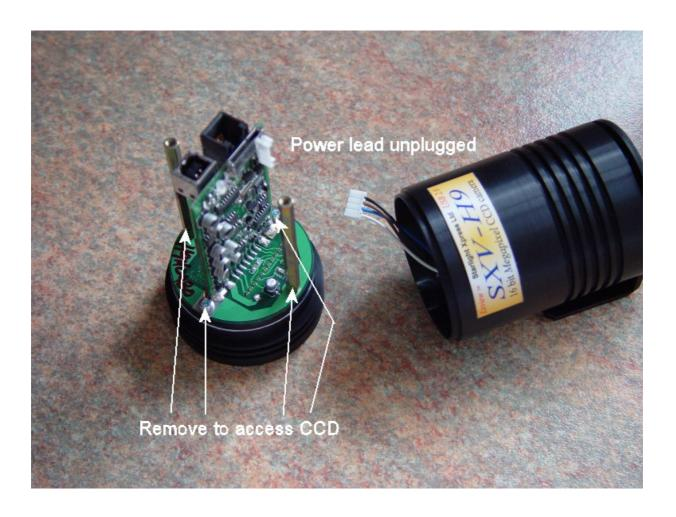
If you only have moisture condensation and no dust to remove, slacken the screws and standoffs as shown, and put the camera in a warm, dry place for a few hours. The moisture will evaporate through the gap and no dust will get onto the CCD:
