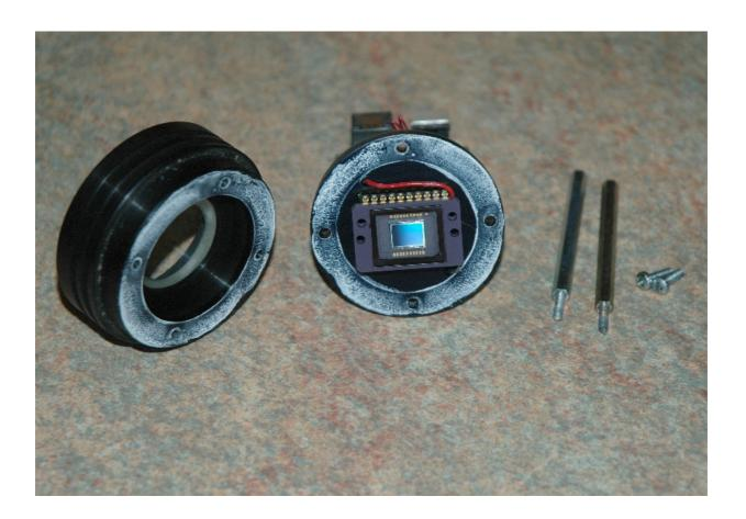
Clean the CCD glass by dropping a few drips of acetone onto it and then gently wiping the microfibre cloth from one end to the other in a single stroke.
