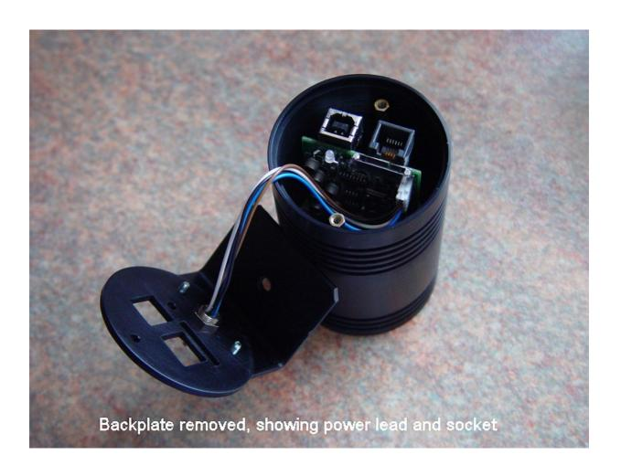
Unplug the power lead from the main board and lift off the main barrel. The long standoffs and screws hold the CCD assembly onto the front barrel:
