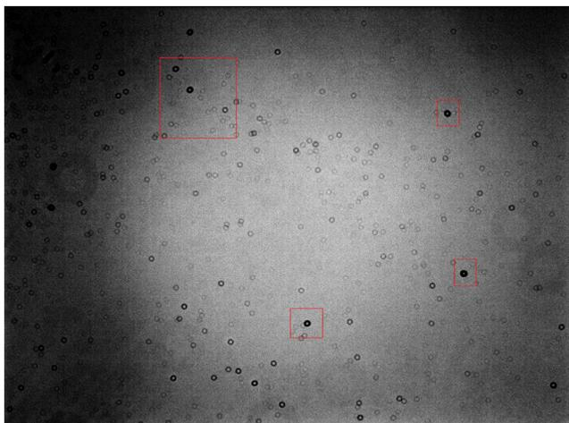
A simple single flat field with red boxes marking the position of large-scale dust on the CCD chip.
