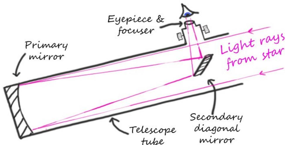
The "Newtonian" reflecting telescope
